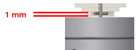
Pic. 13: Mounting the pulley
