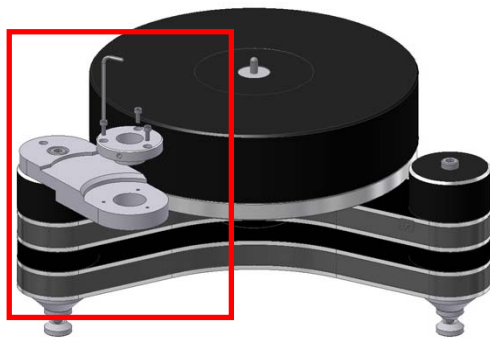
Pic. 7: Placing the tonearm
