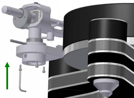
Pic. 3: Set-up of tonearm base with VTA-Lifter
