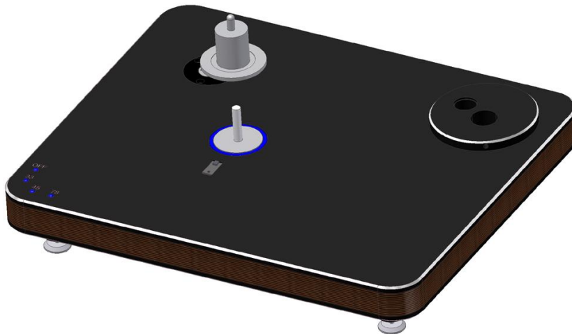
Pic. 4: Fitting the bearing upper part
